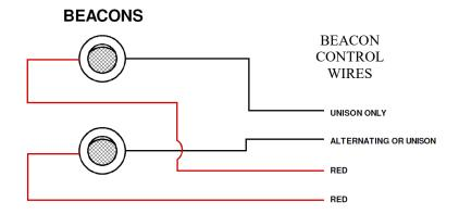
RECOMMENDED WIRING BEACONS 12W OR LESS, 12V DC DISPLAY BEACON TIMING
