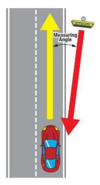
Figure 6-2. Radar Speed Errors
