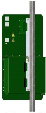
iQ1500 Bolted to Minimum 2.5" Square pole Utilizing Universal Bracket
