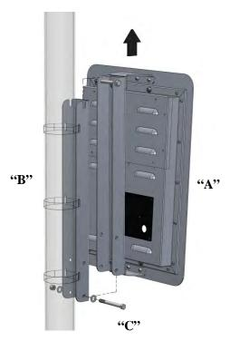
Figure 5-2. Connecting DFB Sign to Bracket
