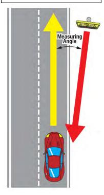
Figure 5-5. Radar Speed Errors
