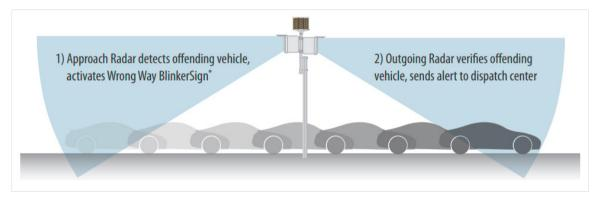
Fig. 2. Dual radar detection and dispatch alert for wrong-way vehicle detection (Traffic and Parking Control Company, 2014)
