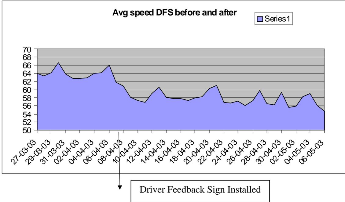
The Driver Feedback Signs had an immediate impact with mean speed reduction and further reduction longer term.
