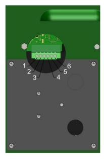
Figure 6-4. External Beacon Connections
