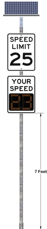
Figure 5-1. Typical DFB Mounting (Solar Panel not present on portable installations)
