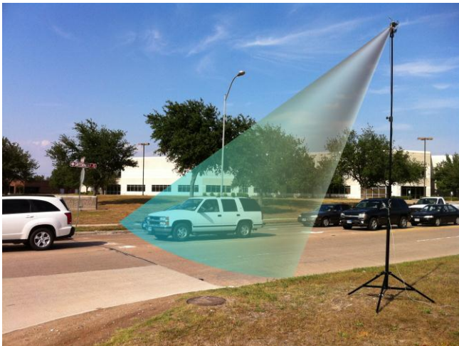
Illustration of PD300/PD310 in side-firing intersection mode with maximum depth of view.
