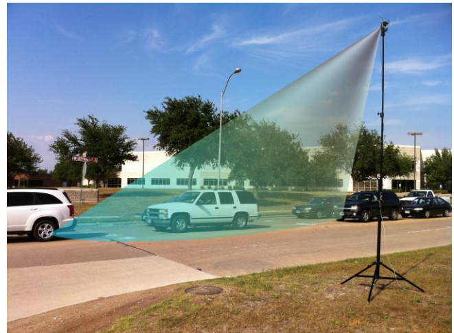
Illustration of rotated PD300/PD310 in side-firing intersection mode with maximum width of view.
