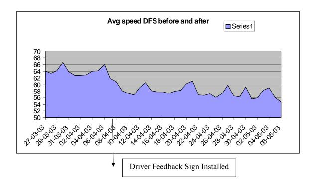
The Driver Feedback Signs had an immediate impact with mean speed reduction and further reduction longer term.
