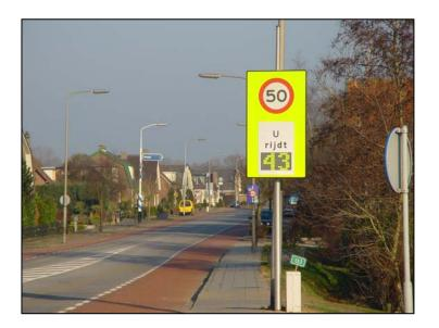
Heesch, Netherlands Evaluation Sign The graph below illustrates speed reductions before and after the Driver Feedback Sign was installed.
