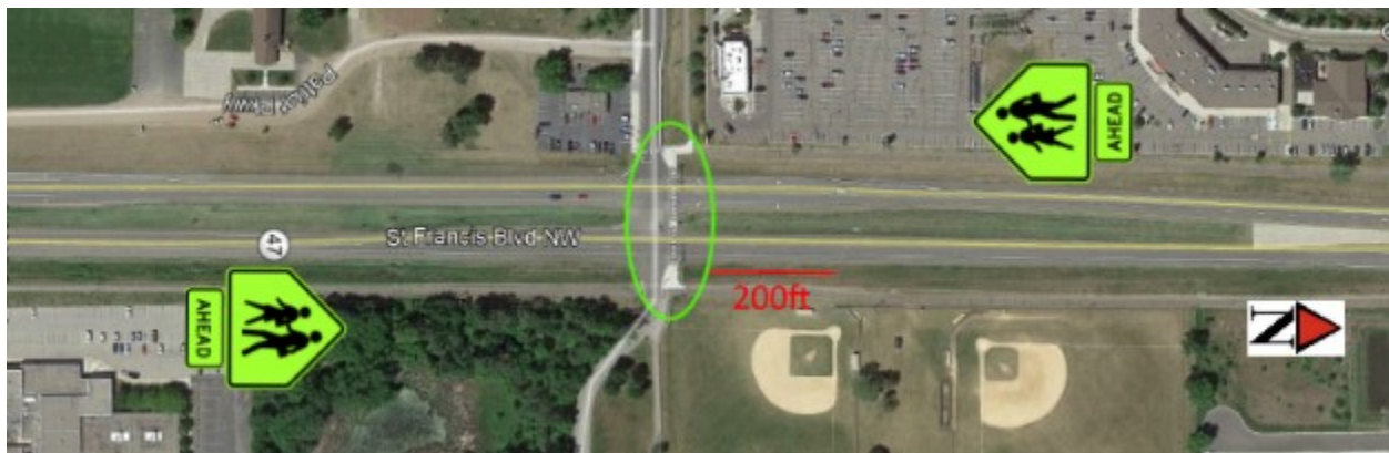
Figure 4-33 Aerial view of Site 26. Advanced warning sign icons correspond to the sign locations. The crossing is highlighted by the green oval.
