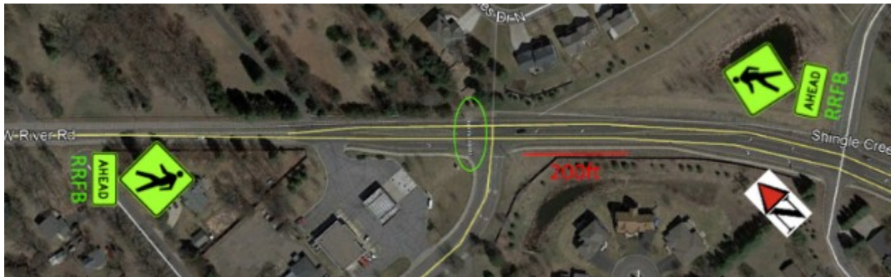
Figure 4-25 Aerial view of Site 12. Advanced warning sign icons correspond to the sign locations. The crossing is highlighted by the green oval.
