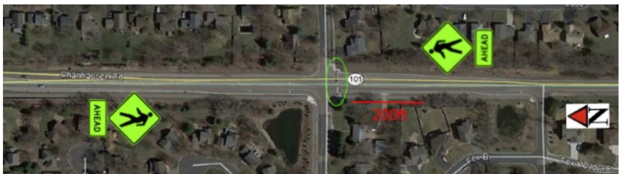
Figure 4-27 Aerial view of Site 23. Advanced warning sign icons correspond to the sign locations. The crossing is highlighted by the green oval.
