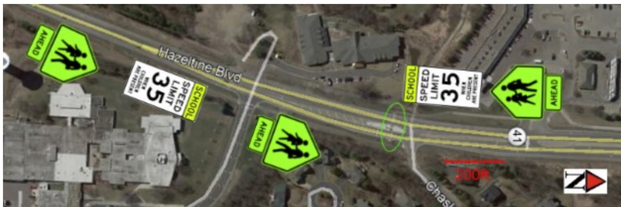
Figure 4-29 Aerial view of Site 24. Advanced warning sign icons correspond to the sign locations. The crossing is highlighted by the green oval.
