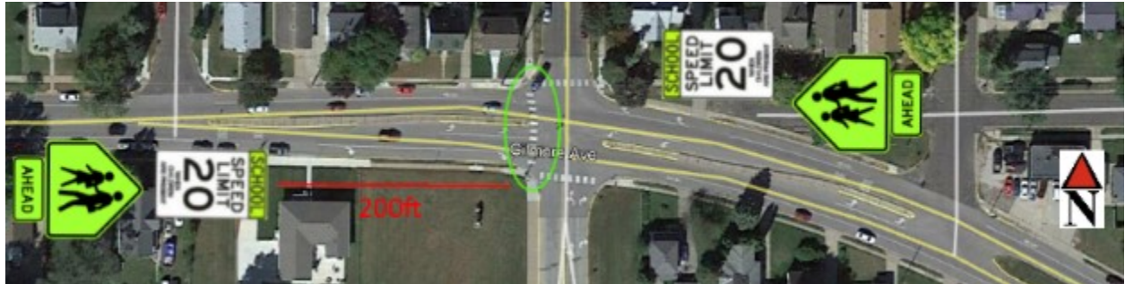
Figure 4-57 Aerial view of Site U4. Advanced warning sign icons correspond to the sign locations. The crossing is highlighted by the green oval.
