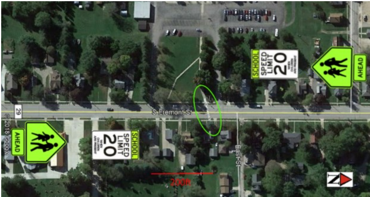
Figure 4-21 Aerial view of Site 4. Advanced warning sign icons correspond to the sign locations. The crossing is highlighted by the green oval.
