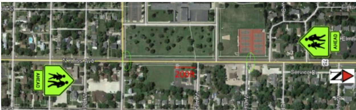
Figure 4-45 Aerial view of Sites 45 (right) and 46 (left). Advanced warning sign icons correspond to the sign locations. The crossing are highlighted by the green oval.
