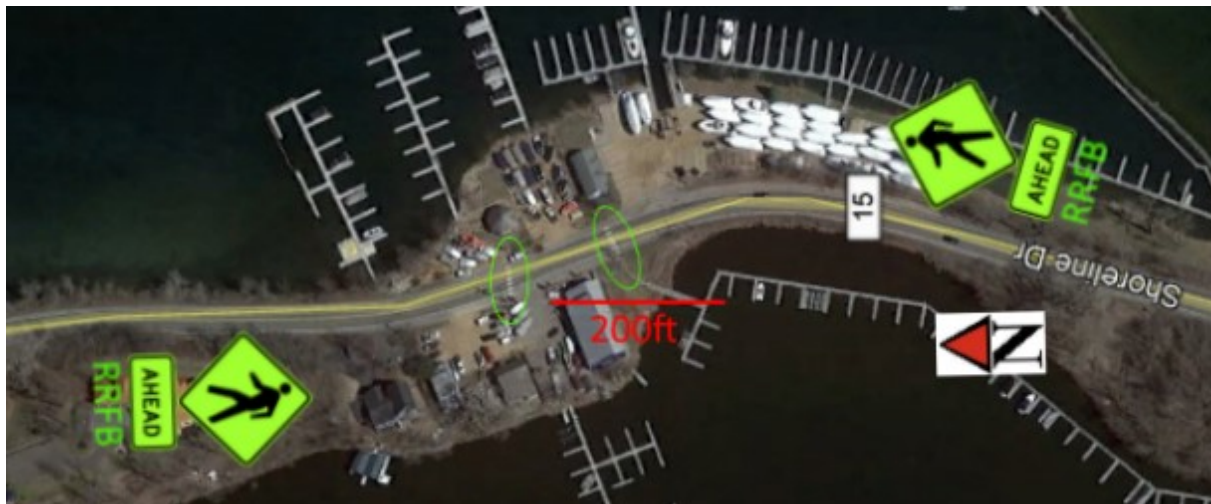
Figure 4-53 Aerial view of Sites U2a (right) and U2b (left). Advanced warning sign icons correspond to the sign locations. The crossings are highlighted by the green ovals.
