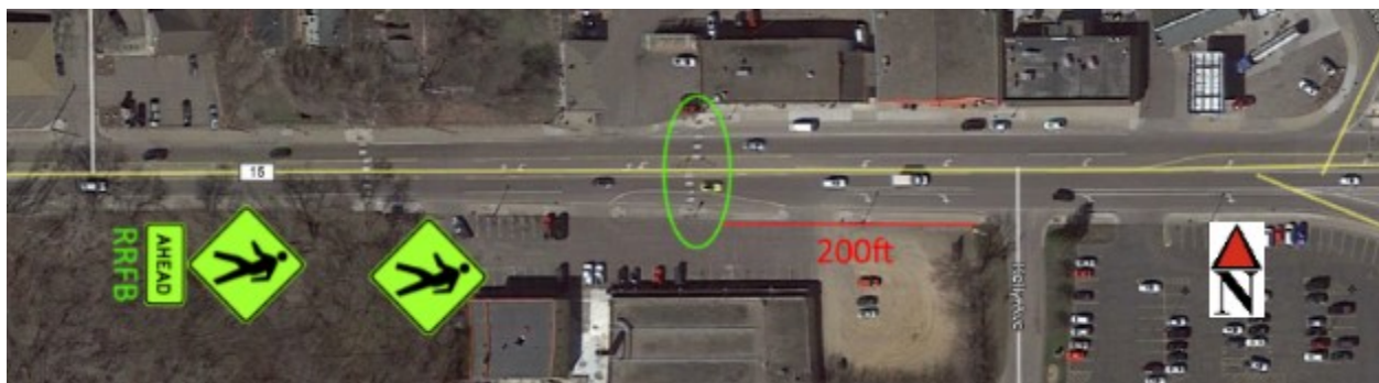
Figure 4-31 Aerial view of Site 25. Advanced warning sign icons correspond to the sign locations. The crossing is highlighted by the green oval.
