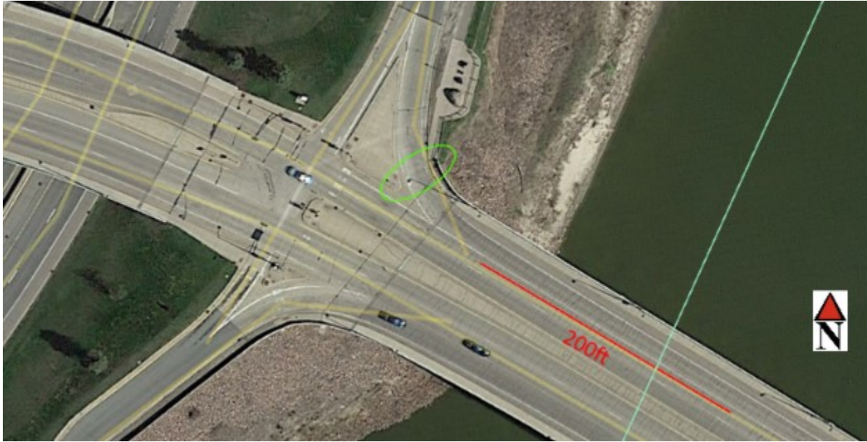
Figure 4-39 Aerial view of Site 38. Advanced warning sign icons correspond to the sign locations. The crossing is highlighted by the green oval.
