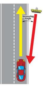
Figure 6-4. Radar Speed Errors
