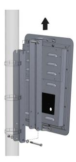
Figure 6-2. Mounting the sign
