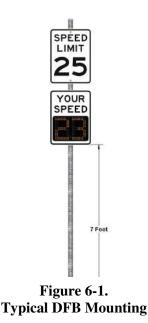
Hang the sign chassis on the hanging bracket on a suitable pole or structure. (See Figure 6-2). Chassis must then be banded and/or anchored/bolted to the mounting structure (Hardware not included).
