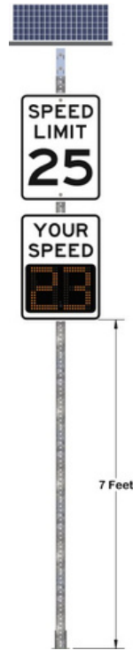
Figure 5-1. Typical DFB Mounting
