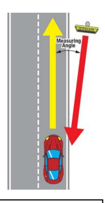
Figure 5-5. Radar Speed Errors
