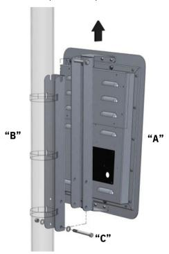
Figure 5-2. Connecting DFB Sign to Bracket
