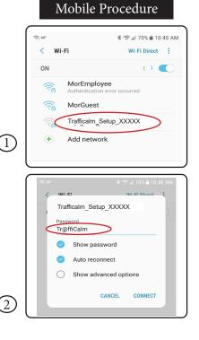
You've now connected to the device's wi-fi. Note that the system does not have Internet connection, so your device will likely not be able to connect to websites, email, or perform other web-required functions. No Internet connection is required to configure the system.
