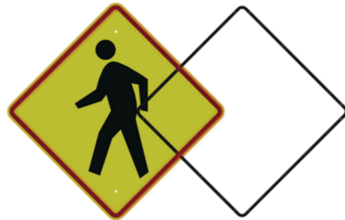
Sign area to clean and prep highlighted
