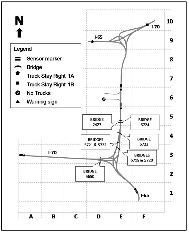
**Figure 9:** Schematic of I-65 – I-70 merger location in Indianapolis, IN and proposed OVD&W system deployment plan (Illustrative – see Google Earth rendering in Appendix for details).
