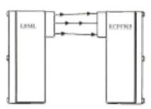
Through beam detection is generally considered better than retro or proximity detection because of greater sensing range and freedom from false detection of shiny objects. However, because of difficulty in alignment and the necessity of locating a separate light source, this method of detection is not used as often.
