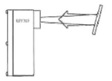
A retro-reflective control generally provides a surer, simpler and more positive detection in applications where a reflector can be used.
