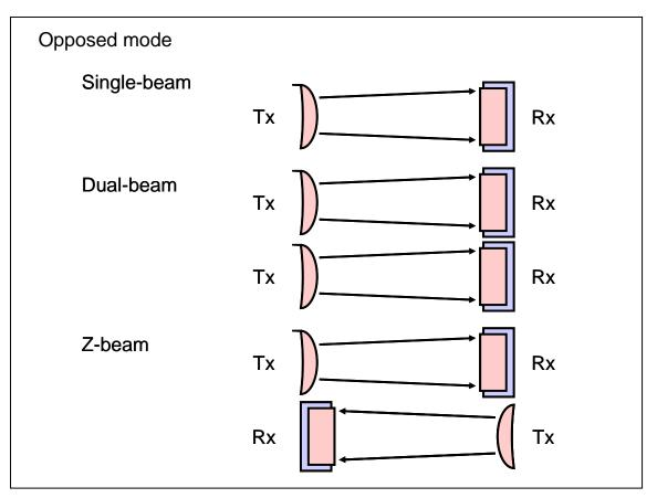
Figure 4: Optoelectronic designs for an opposed mode system.
