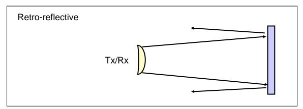
Figure 4: Retro-reflective operational configuration of infrared optoelectronic sensor.
