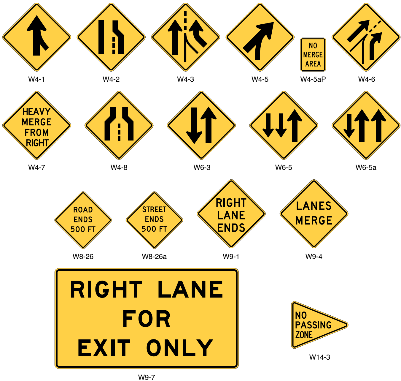
Figure 2C-11. Merging and Passing Signs and Plaques
