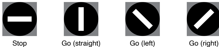
Figure 8D-3. Light Rail Transit Signal Indications
