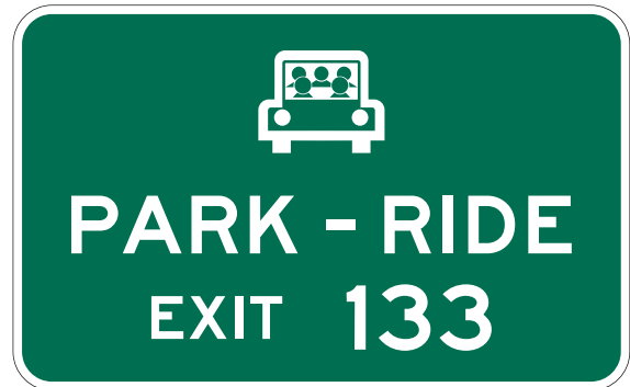
Figure 2E-54. Examples of Supplemental Guide Signs for a Park-and-Ride Facility
