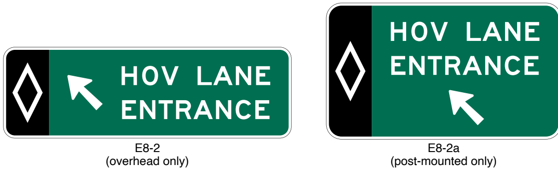
Figure 2G-6. Examples of Overhead or Post-Mounted Preferential Lane Entrance Direction Signs
