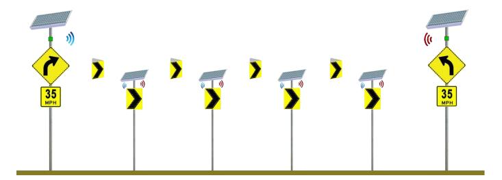
Installed firmware at each Chevron location allows systems operating on bi-directional roadways to work autonomously and independently of one another and provide multi-directional transmitting.
