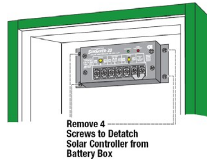
Figure 3-2. Remove Solar Charger from Battery Box
