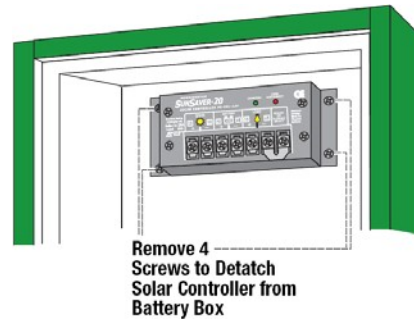
Figure 3-2. Remove Solar Charger from Battery Box
