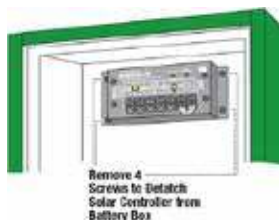
Figure 3-2. Remove Solar Charger from Battery Box
